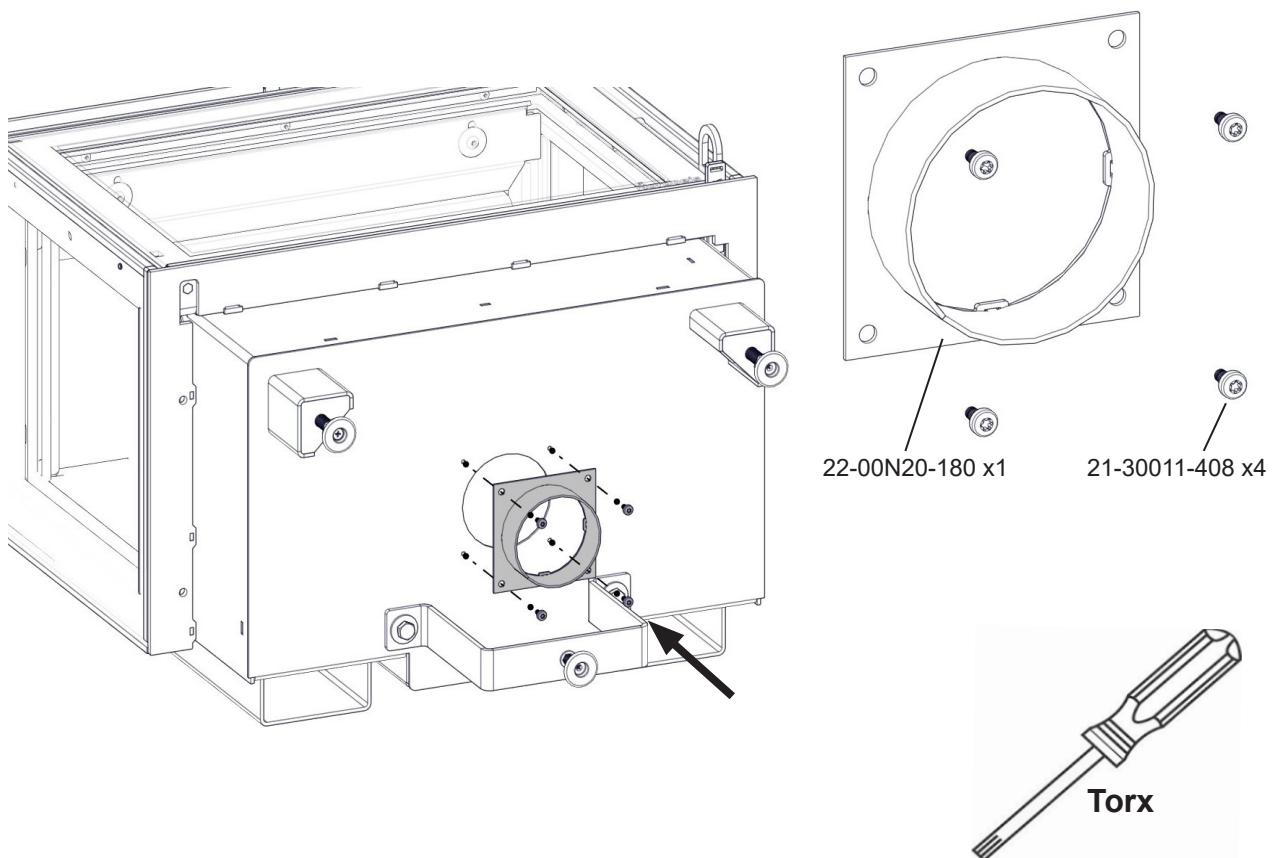
**FIG 4a** Air inlet adapter 90° assembling - optional
