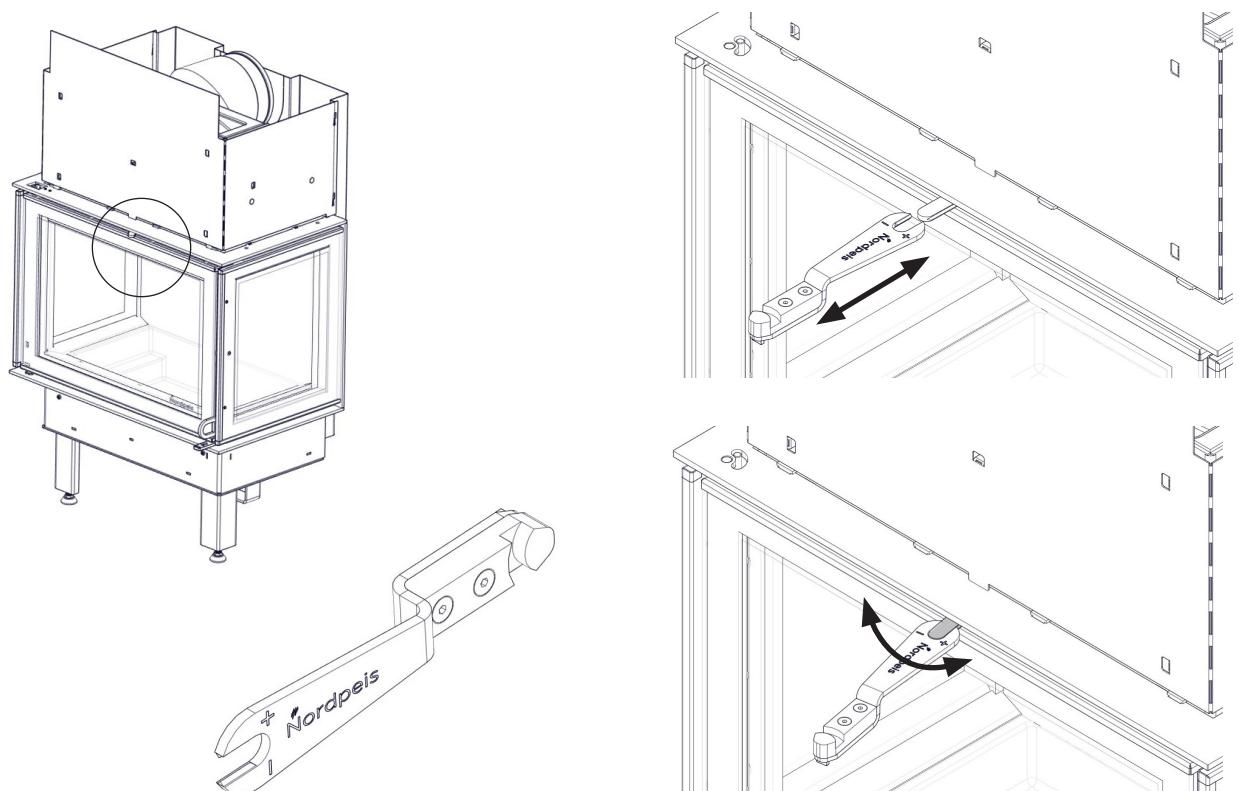
**FIG 8c** Operational handle - door opening usage
