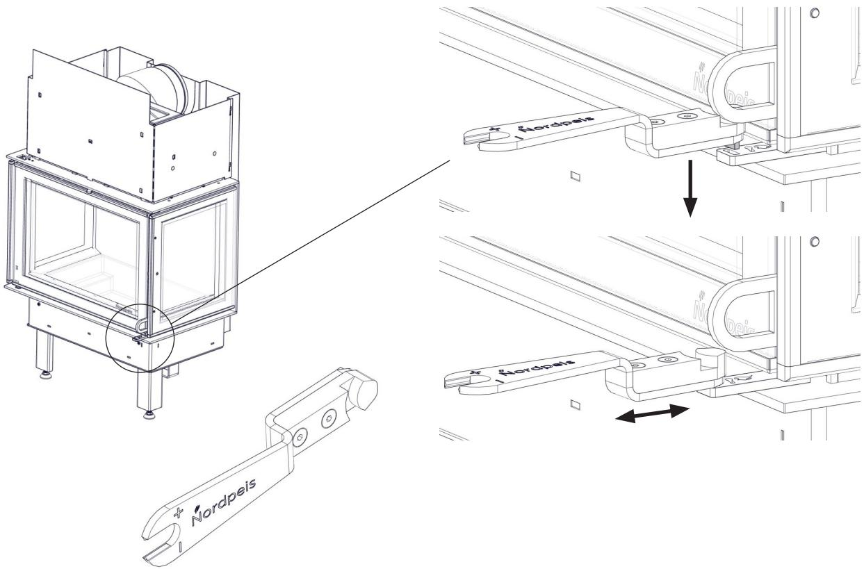
**FIG 8b** Operational handle - secondary valve usage
