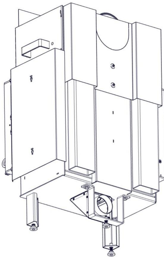
**FIG 5** Smoke adapter - rear chimney connection
