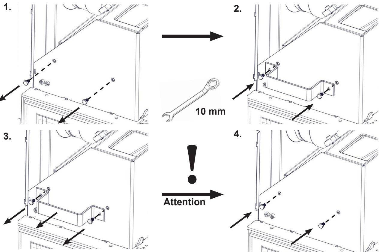
**FIG 7** Front radiation shield - assembling
