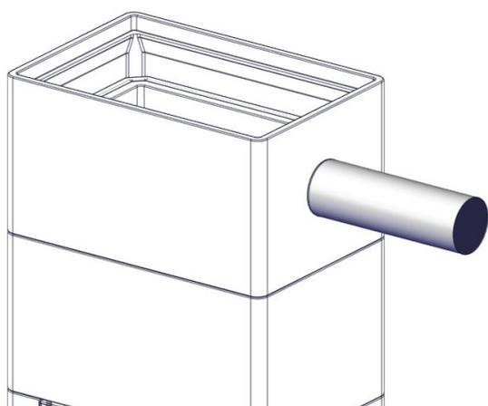
Place the smokepipe. Before placing the next Powerstone, make sure the connection between the Powerstone and the smokepipe is sealed. The flue pipe should be flush with the inside of the Powerstone.
