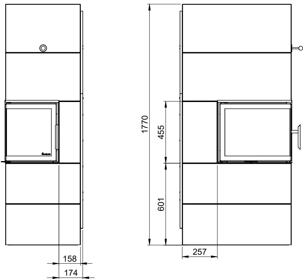
**GB** In case that the fireplace is placed freestanding without the heat shield in the back, the minimum distance behind to combustible material is 800mm.
