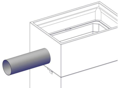
Place the smokepipe. Before placing the next Powerstone, make sure the connection between the Powerstone and the smokepipe is sealed. The flue pipe should be flush with the inside of the Powerstone.
